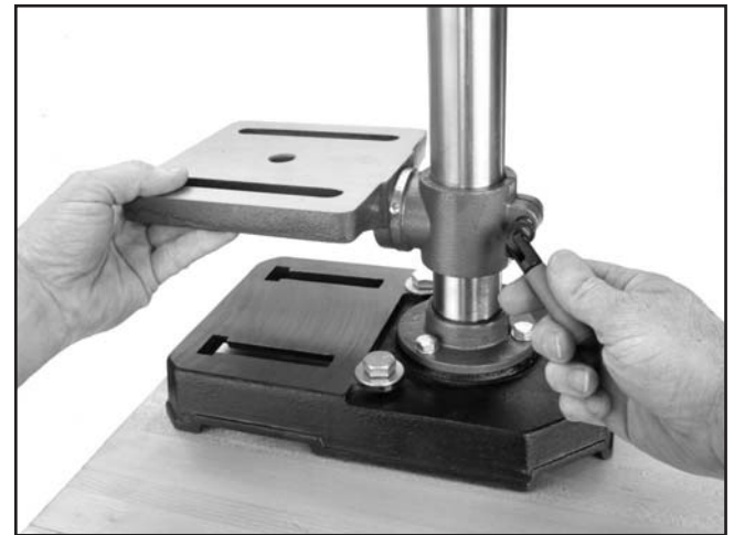
Figure 10. Securing table support.
